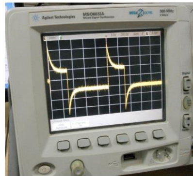
Fig. 6(b) The obtained actual waves shape from the pacemaker.
